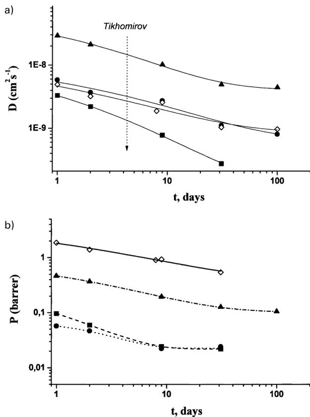
Fig. 1. Time dependence of the diffusion coefficients (a) and permeability (b) of  $\text{O}_2$  (▲),  $\text{N}_2$  (●),  $\text{CO}_2$  (◇) and  $\text{CH}_4$  (■) in PVC.
