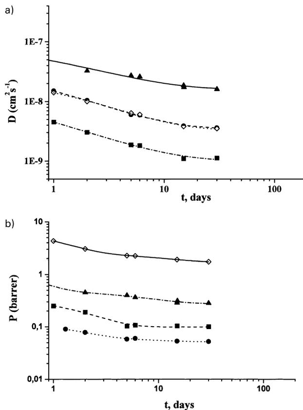
Fig. 2. Time dependence of the diffusion coefficients (a) and permeability (b) of  $\text{O}_2$  (▲),  $\text{N}_2$  (●),  $\text{CO}_2$  (◇) and  $\text{CH}_4$  (■) in PVC-pyr7.
